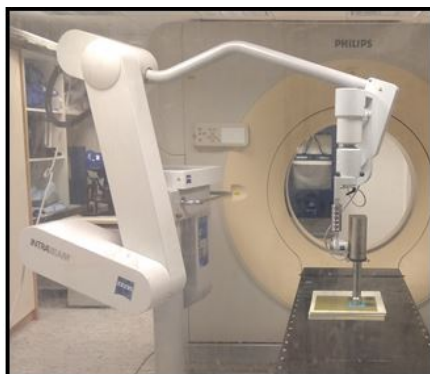
Figure 1: The Carl Zeiss INTRABEAM®-system a mobile intraoperative x-ray device during measurement.
