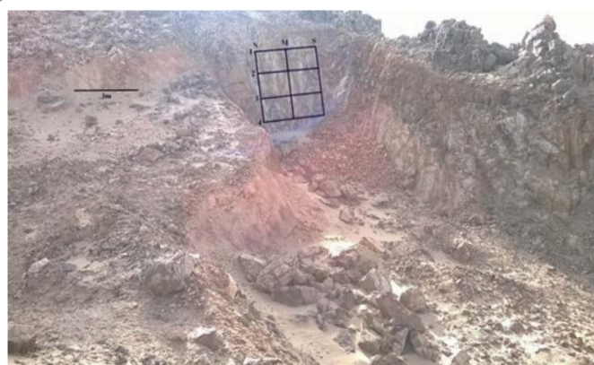
Figure 2 A grid pattern on the vertical granitic face to investigate the concentrations of U, Th and K. The picture was taken looking east.
