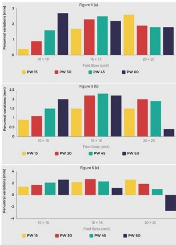
**Figure 3:** Represents variations in penumbral width in presence of virtual wedge for 15 MV energy (a) D<sub>max</sub> (b) 10 cm (c) 20 cm.
