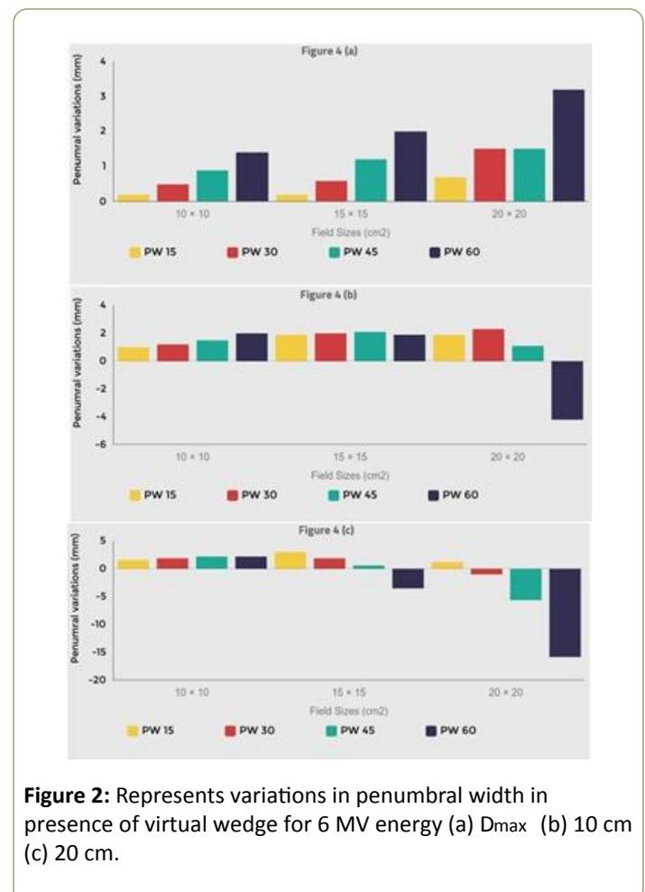
**Figure 2:** Represents variations in penumbral width in presence of virtual wedge for 6 MV energy (a) Dmax (b) 10 cm (c) 20 cm.
