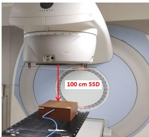
**Figure 3:** RMI 457 Solid water set-up.
