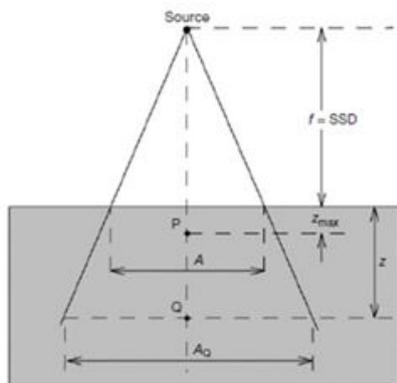
**Figure 1:** Percentage Depth Dose (PDD) measurement set-up (Adapted from Podgorsak E.B. Radiation Oncology Physics: A Handbook for Teachers and Students, IAEA, 2005:186).
