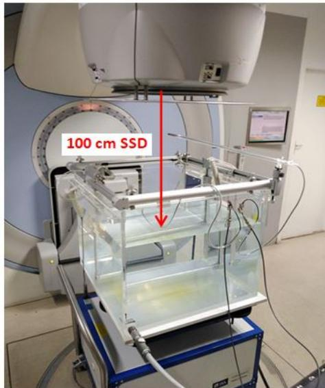
**Figure 2:** Water phantom set-up.
