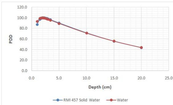
**Figure 6:** PDDs for RMI 457 and water phantoms for 8 MV.
