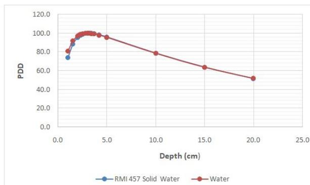
**Figure 7:** PDDs for RMI 457 and water phantoms for 18 MV.
